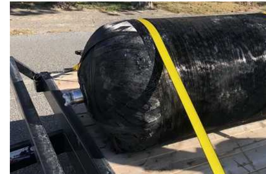
SpaceX Falcon 9 helium tank recovered from a farm in Washington state (March 2021)
