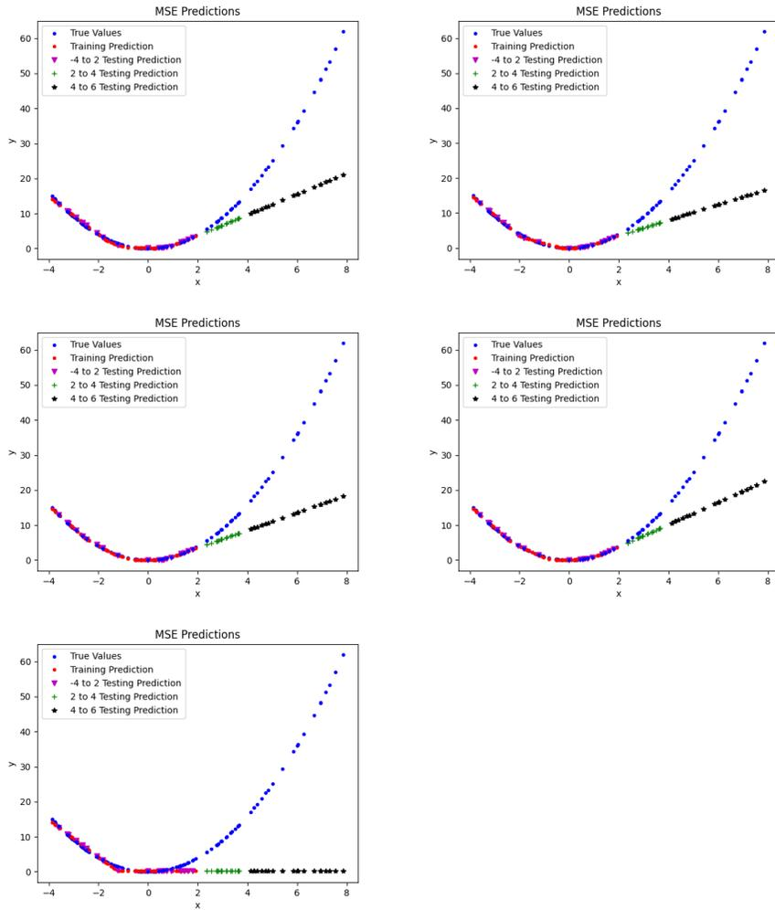
Figure 2: Behaviors of trials 1 to 5 predicted with a neural network model and MSE loss function
