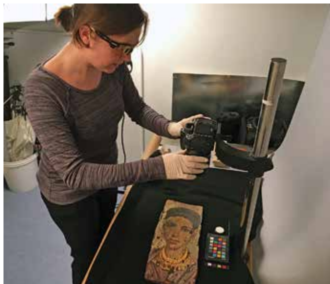
Carrie performing visible-induced infrared luminescence imaging on the Fayum portrait using a modified DSLR camera. Photo by Amaris Sturm.
