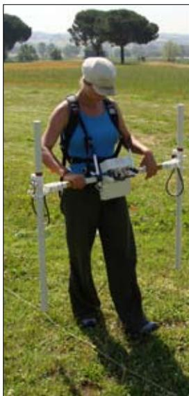
Fig. 2. Magnetometry in progress.
