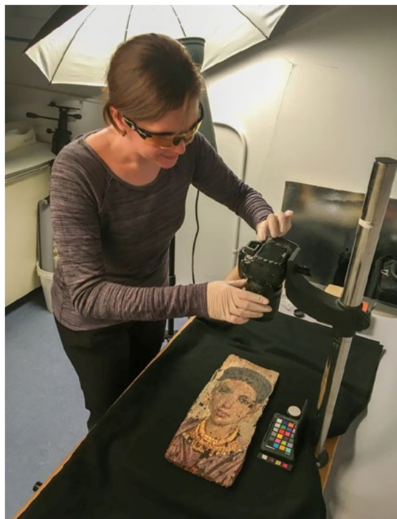
Investigating ancient color. Carrie Roberts performs multispectral imaging (MSI) on a mummy portrait from the Fayum region of Egypt. Photo by Amaris Sturm.
