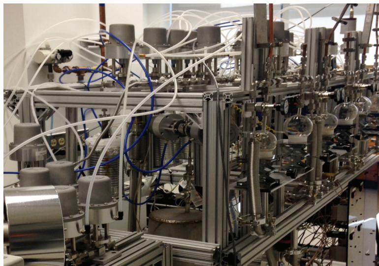
Automated system for the extraction of noble gases from waters and natural gases was developed in the Noble Gas Laboratory at the University of Michigan.
