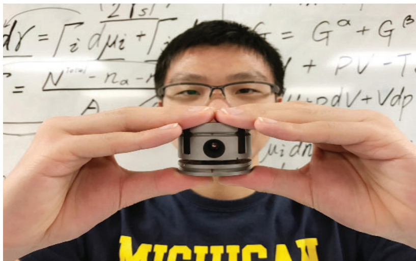
Junjie Dong, a senior student, holds a diamond anvil cell, which enables researchers to simulate Earth's extreme ranges of pressure and temperature in the laboratory. He is now pursuing his PhD at Harvard University.
