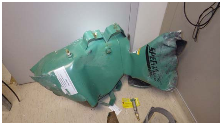
Below—Photo of tank after explosion by Honolulu Fire Department
