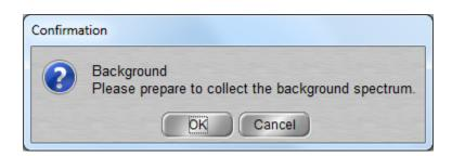
3. After confirmation, the instrument begins to collect data. The steps that the instrument takes can be viewed in the bottom left corner of the screen. First, a couple of setup processes are completed, then a countdown of the chosen number of scans begins (1 of 8, 2or 8, etc.). When the collection is complete, the spectrum is displayed and you are prompted to save the data to the currently opened window. If the data are acceptable, click "Yes" to save the spectrum.
