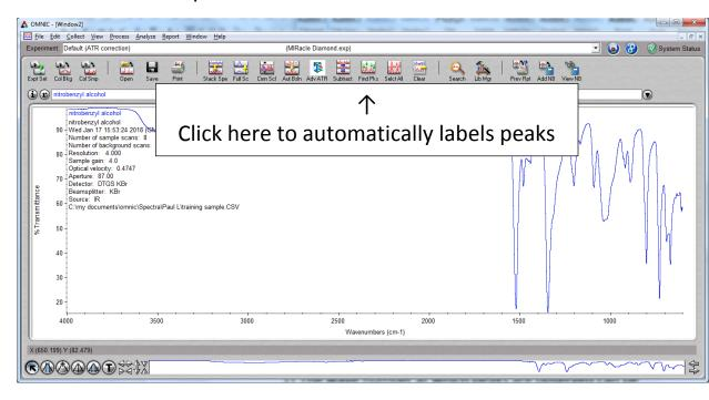
2) When the Find Peaks button is clicked, a horizontal line appears on the spectrum, indicating the threshold value for defining a peak. Click with the tip of the cursor to reposition this threshold line. When the desired position is determined, click on the Replace button in the upper right corner of the page to lock in the threshold value.
