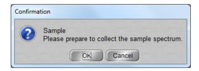
5. After confirmation, the instrument begins to collect data. The steps that the instrument takes can be viewed in the bottom left corner of the screen. First, a couple of setup processes are completed, then a countdown of the chosen number of scans begins (1 of 8, 2or 8, etc.). When the collection is complete, the spectrum is displayed and you are prompted to save the data to the currently opened window. If the data are acceptable, click "Yes" to save the spectrum.
