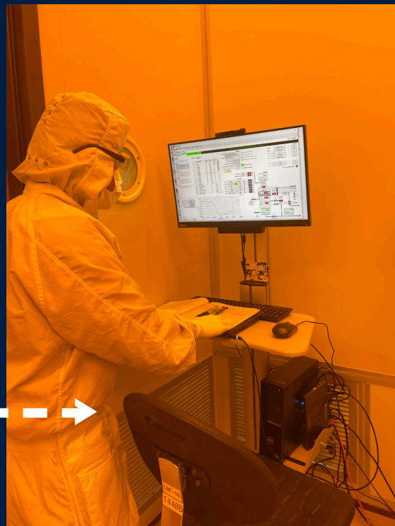
He uses the computer interface to control the ALD reactor, specifying the “recipe” and parameters he is interested in manipulating.
