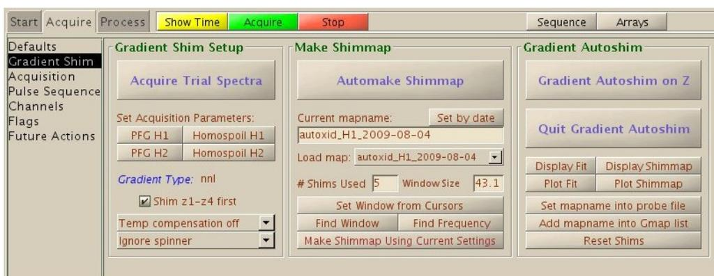
The first step is to make sure an appropriate shim map is already loaded under the Current mapname: field. Map names are made up of the probe name, followed by the nucleus (lk or H1), followed by the date, for example: autoxid\_H1\_2009-08-04. If a proton map is not already loaded, select the most recent map available for H1 shimming from the Load map: drop down menu.
