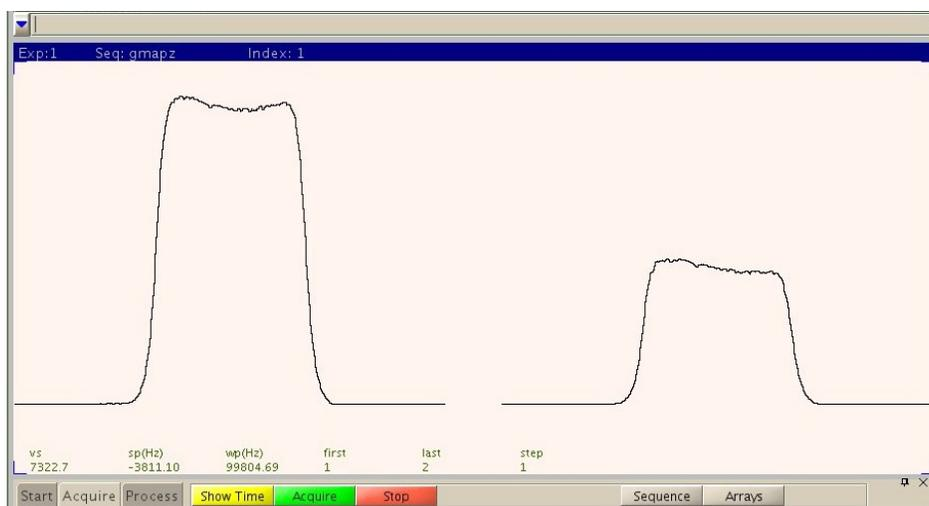
After adjusting parameters, click [Gradient Autoshim on Z]. The shimming process then starts and after each iteration, it displays a plot of the magnetic field homogeneity similar to the one shown below. A successful shimming should show a red curve that is as flat and horizontal as possible. Some noise or deviation at the edges is common. If not satisfied, the shimming process can be repeated. To finish, click [Quit Gradient Autoshim].
