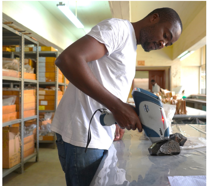
James K. Munene tries out a portable X-ray fluorescence (pXRF) analyzer at the National Museums of Kenya. Photo by John Munyiri.
