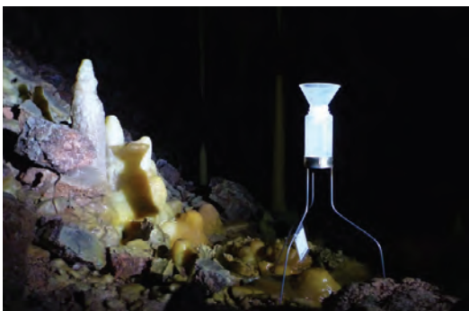
Monitoring cave dripwaters helps us understand our records better. Here in Kartchner Caverns State Park, AZ, water samples are collected monthly for isotopic and geochemical analysis.
