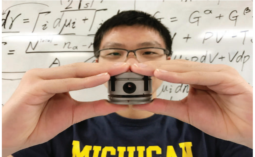
Junjie Dong, a senior student, holds a diamond anvil cell, which enables researchers to simulate Earth's extreme ranges of pressure and temperature in the laboratory. He is now pursuing his PhD at Harvard University.
