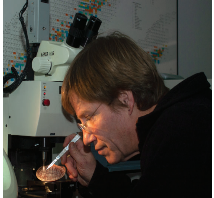
Kacey Lohmann (Professor) removing powder carbonate sample to reconstruct seasonal-scaled isotopic temperatures for an Antarctic scallop using the Micromill Microsampler. This device was developed in collaboration with MerchanteK based on a prototype developed by Kacey and David Dettman (PhD '91).
