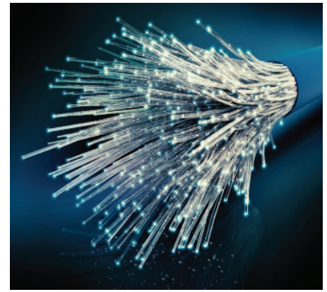
Fiber Optic Cables become the new seismometer. Changes in backscattered light reflects how the fiber stretches and compresses in response to seismic waves.
