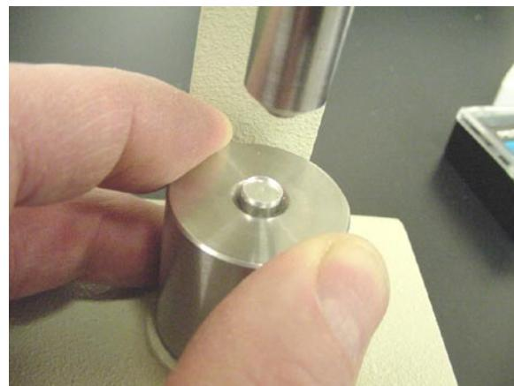
5) Push down on crimping tool to crimp the sample pan shut.
