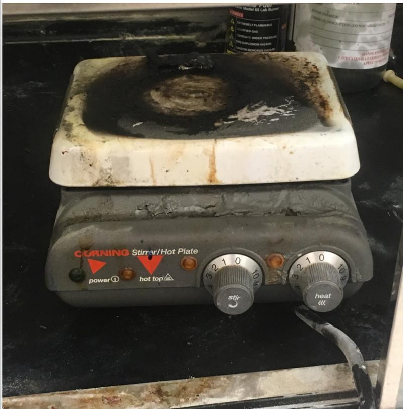
This fire appears to have been caused by what is known as a “runaway” hotplates. This occurs when malfunctions in certain models of hotplates cause them to spontaneously heat up when they are in the OFF position. This primarily occurs in older models that do not have temperature feedback controls.
