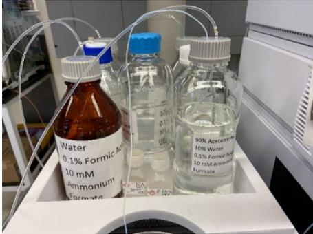
If the acetonitrile bottle is low on solvent, please replace the bottle with one of the spare full bottles of acetonitrile. Then update the solvent level in the software so that the data system will know how much solvent is available.
