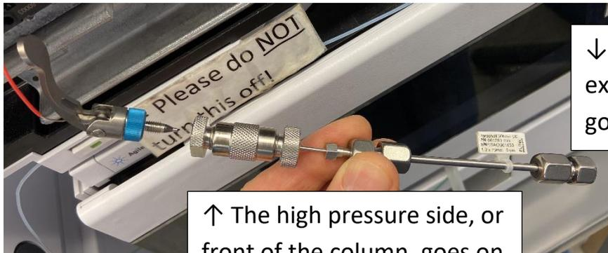
↑ The high pressure side, or front of the column, goes on the left side.
