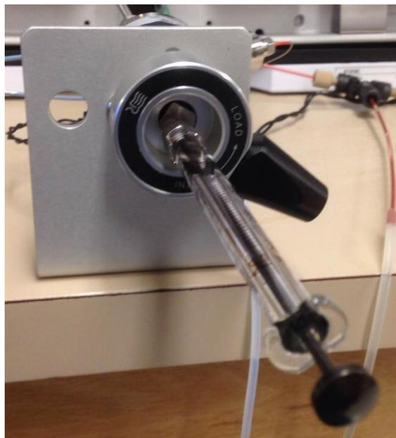
↓ Rotate handle down to start the run.
