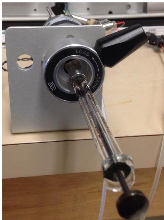
↑ Handle still up in Load position while injecting the sample solution.
