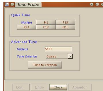
Unfortunately, the protune unit is notoriously unreliable. It usually does a good job, especially for  $^1\text{H}$ ,  $^{19}\text{F}$  and  $^{13}\text{C}$ , but for other nuclei it may fail. This is especially true for some nuclei like  $^{11}\text{B}$  and  $^{199}\text{Hg}$  in our 400-MR spectrometers *Cobalt* and *Gallium*. If automatic tuning fails
