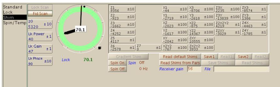
Broad, symmetrical peaks indicate that Z1 and Z3 need optimization while asymmetrical peaks with long tails or shoulders on either side indicate faulty Z2 or Z4 settings. The
