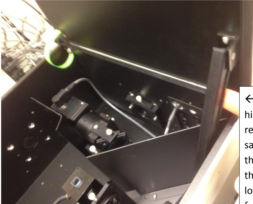
← push back of hinge out to release the safety lock on the hinge so that the door can be lowered from the full open position
