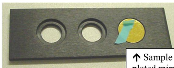
↑ Sample is shown on gold-plated mirror on microscope slide.
