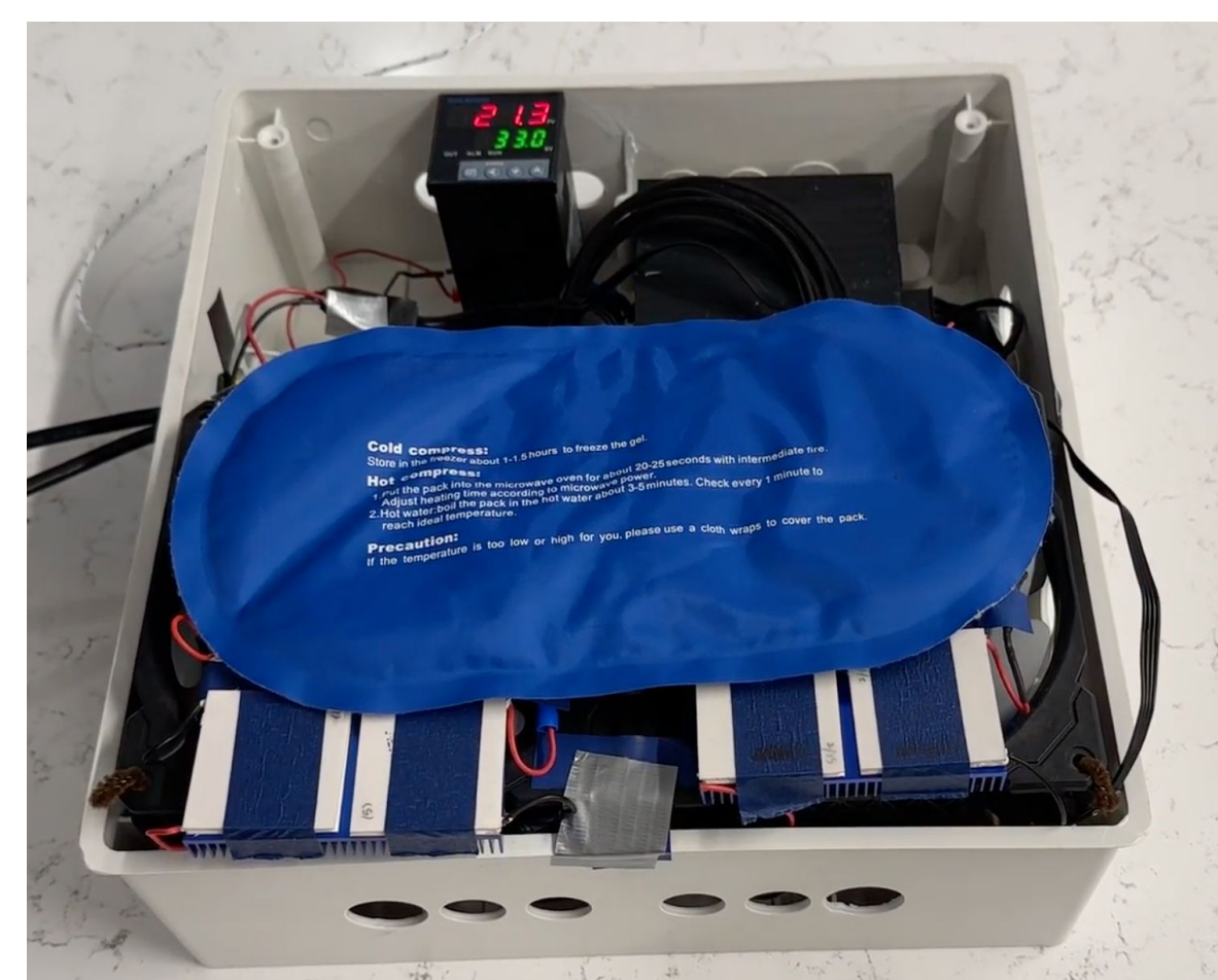
Fig. 4: Testing of gel mattress atop cooling system
